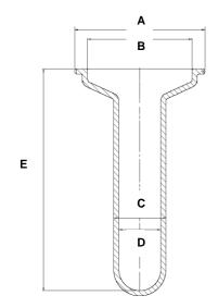
Outside Ø + 0.3 / - 0.2 mm Dimensions: 124.5 mm Α В Inside Ø ± 0.5 mm 100.0 mm C Outside Ø ± 1.0 mm 50.0 mm D Inside Ø 40.0 mm ± 1.0 mm Е Height 211.5 mm ± 0.5 mm
