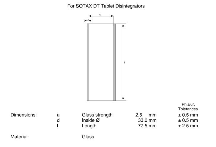
The accuracy of the above mentioned part dimensions have been examined. All relevant measurements are within tolerance and the factory acceptance test has passed. The dimensions are in conformance with Ph. Eur. 2.9.1.-2 Pharmacopeia requirements (at time of delivery).
