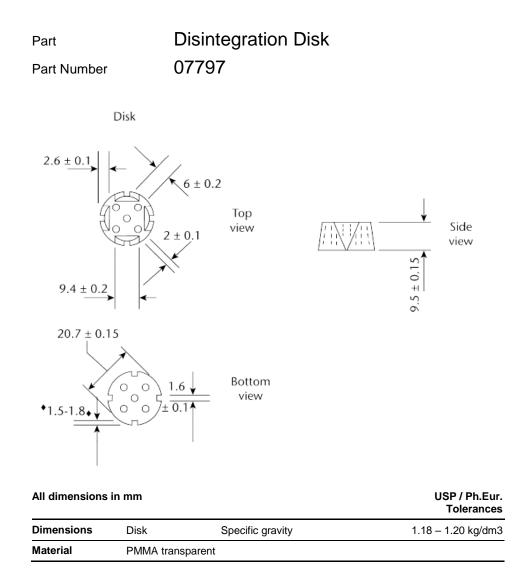
The accuracy of the above mentioned part dimensions have been examined. All relevant measurements are within tolerance and the factory acceptance test has passed. The dimensions are in conformance with USP and Ph. Eur. Pharmacopeia requirements (at date of approval, see below).
