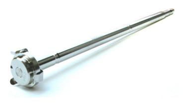
Tolerances Dimensions: Shaft Ø 9.4 to 10.1 mm - -Cap Ø 25.0 mm ± 3.0 mm Cap size 5.1 mm ± 0.5 mm Clear opening 20.2 mm ± 1.0 mm Vent hole Ø 2.0 mm ± 0.5 mm
