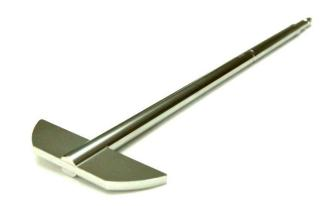
Tolerances Dimensions: Paddle Height 19.0 mm ± 0.5 mm Upper length 74.5 mm ± 0.5 mm Lower length 42.0 mm ± 1.0 mm Size 4.0 mm ± 1.0 mm Radius 1.2 mm ± 0.2 mm Radius 41.5 mm ± 1.0 mm Shaft 9.4 to 10.1 mm Diameter
